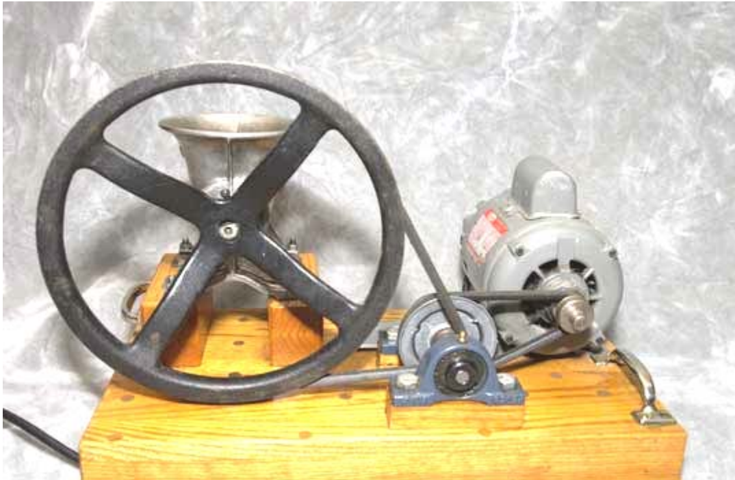
THIS REAR VIEW SHOWS THE RELATIONSHIP OF FLYWHEEL, SPEED BRAKE AND MOTOR.
